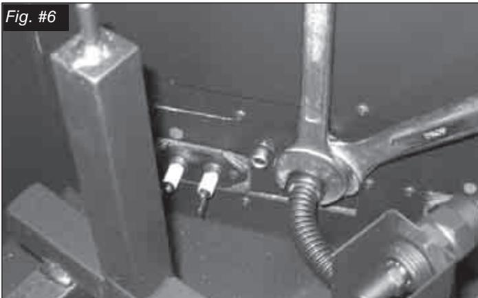
6. Attach the manifold supply tube from the upper burner to the rear bulk head fitting and tighten. (Fig. # 6) Ensure that there are no leaks.
