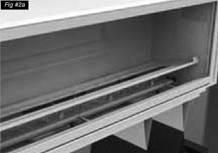
2. Tilt burner tray length-wise and insert into the firebox. Be sure pilot is attached to burner support rail with screw in first hole position. (Fig. #2a & 2b)
