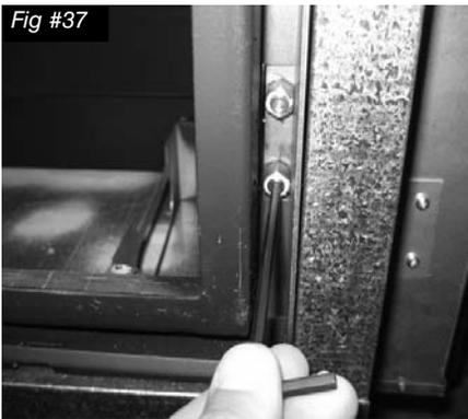
1. Remove the plug from the pressure test port using a 3/16" hex key. The plug is located between the right side lintel and firebox side. (Fig. #37)
