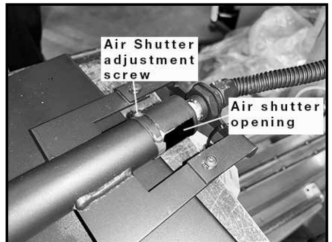
Figure 28: Shutter set for propane.
