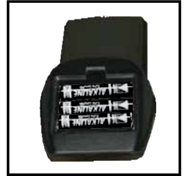
Figure 6: Proflame 2 remote control battery bay.
