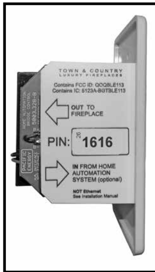
Figure 20: Wall switch with PIN number.
