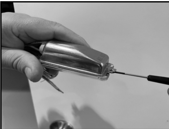
Figure 34: Insert small flat screwdriver.
