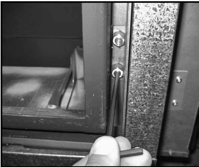
Figure 20: Removing blanking plugs.
