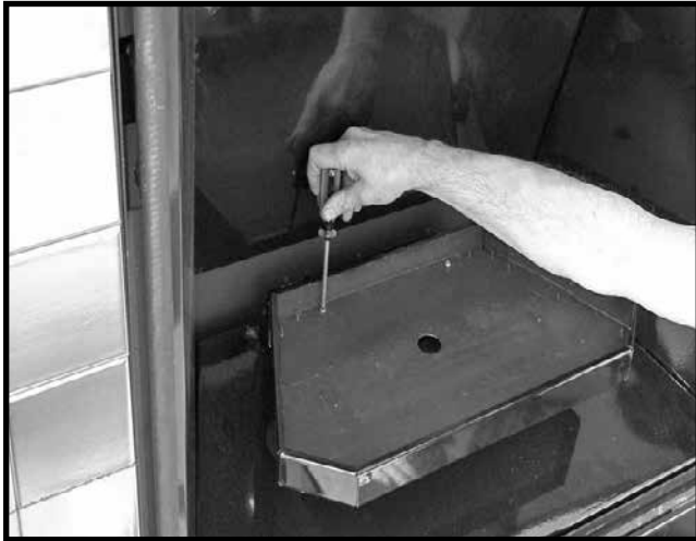
Figure 19: Attaching burner tray to burner shield.
