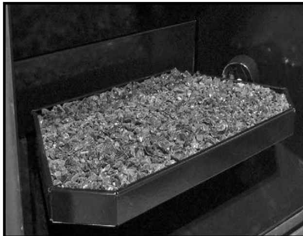
Figure 27: Burner covered with glass media.
