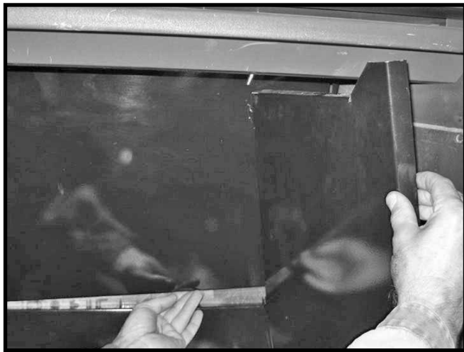
Figure 13: Installing upper rear panel.
