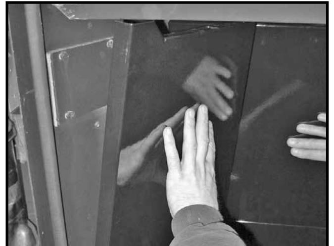
Figure 14: Positioning the left hand side panel.
