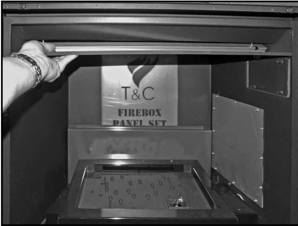
Figure 12: Panel retainer removal.
