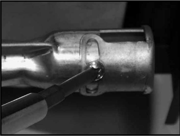
Figure 32: Air shutter half opened for propane gas.
