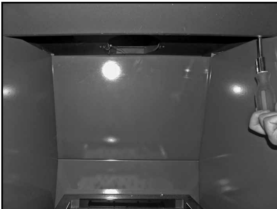
Figure 17: Panel retainer reinstalled.
