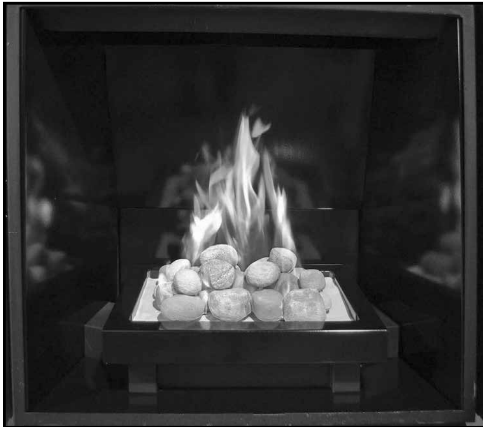
Figure 41: Desirable flame appearance.
