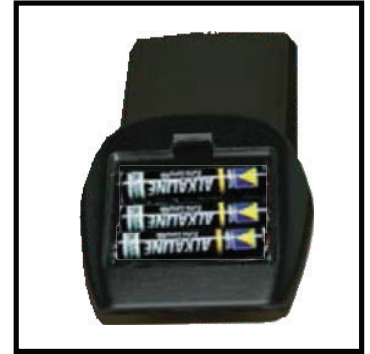
Figure 61: Proflame 2 remote control battery bay.
