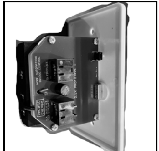
Figure 29: Basic wall switch - interface side.
