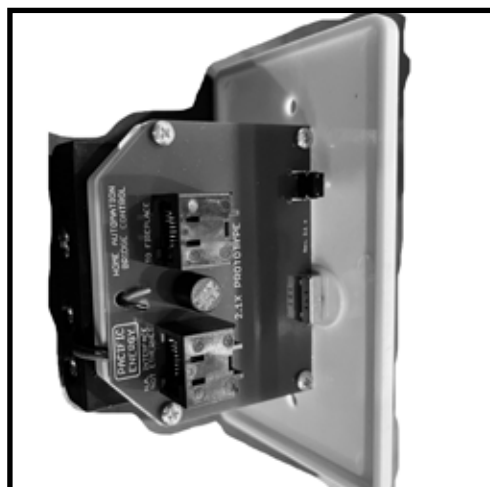
Figure 29: Basic wall switch - interface side.
