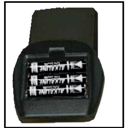
Figure 6: Proflame 2 remote battery compartment.
