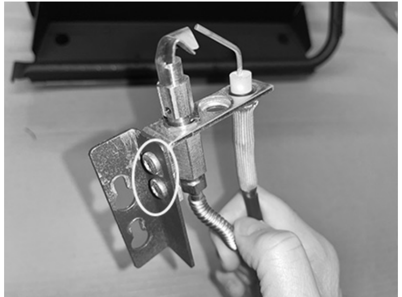
Figure 45: Attach pilot mounting bracket to Unit pilot.
