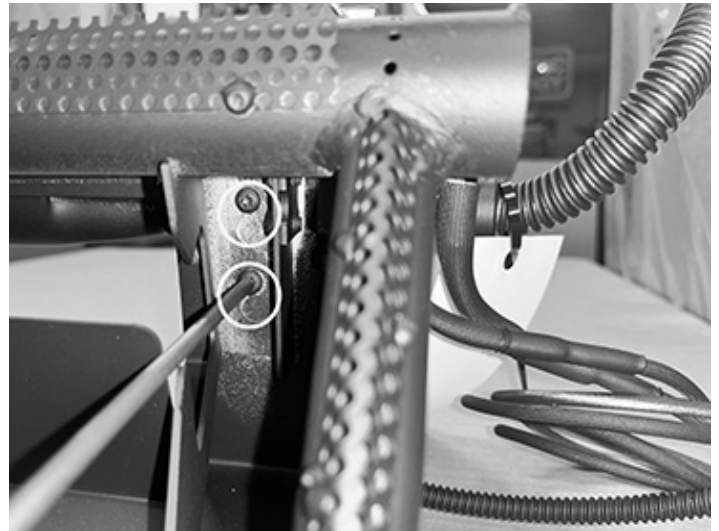
Figure 43: Remove burner pilot.
