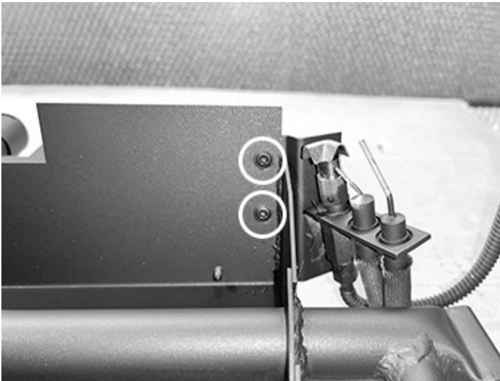
Figure 42: Remove burner pilot.
