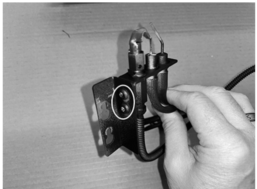
Figure 44: Remove pilot mounting bracket.
