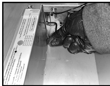
Figure 25: Releasing gas valve assembly from main body.
