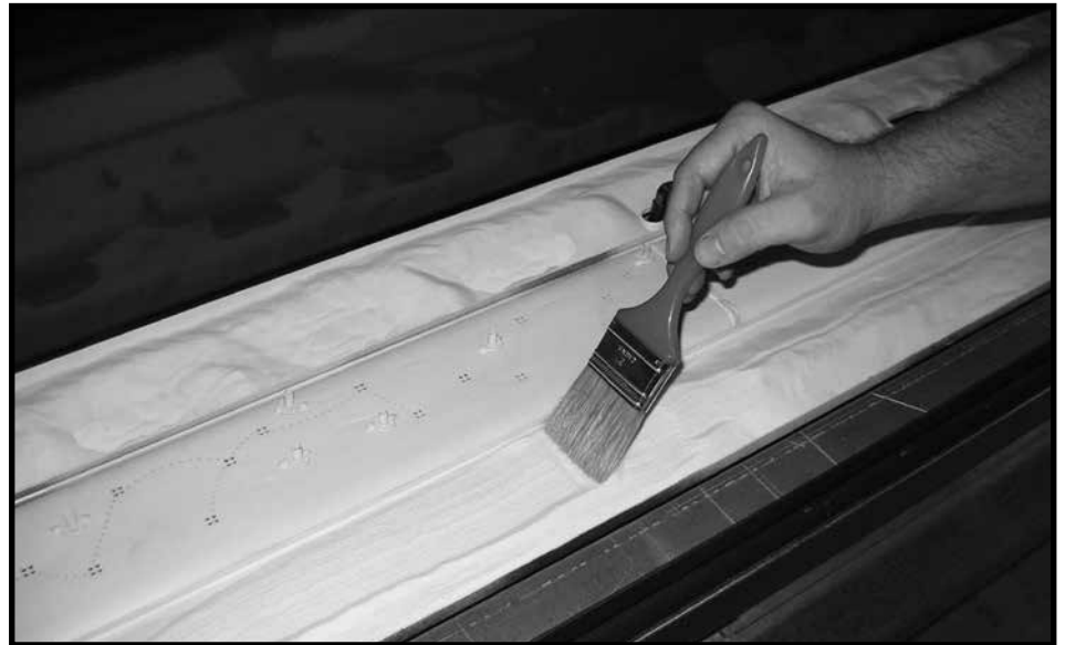
Figure 49: Smoothing sand with brush.
