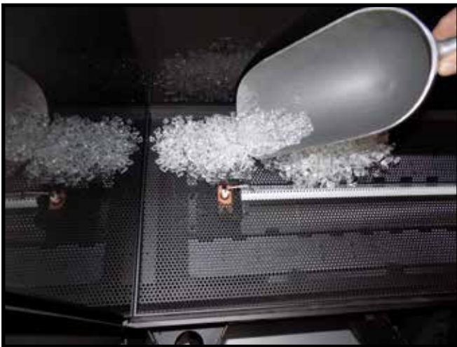
Figure 41: Applying crushed glass on burner tray.
