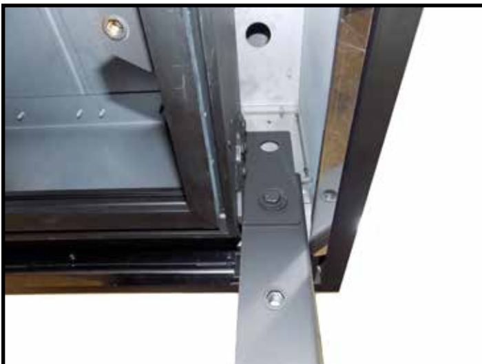
Figure 9: Vertical support upper bolt to be removed.
