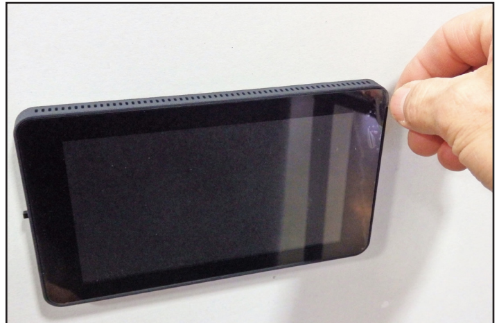
Figure 9: Protective Film Removal
