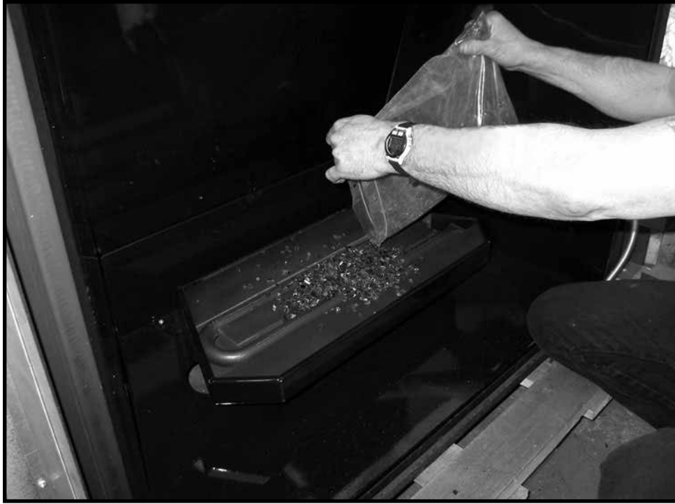
Figure 21: Applying glass media.
