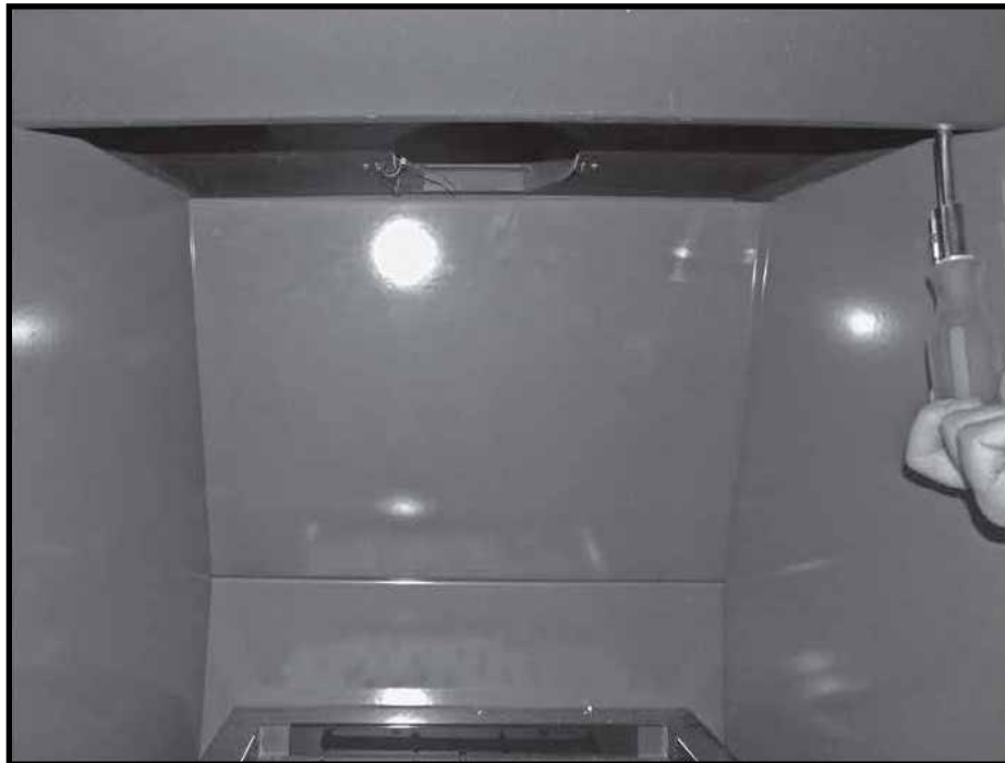
Figure 21: Panel retainer reinstalled.
