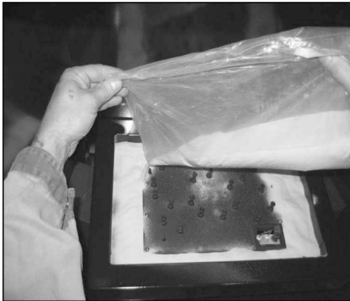
Figure 24: Applying sand to burner tray.
