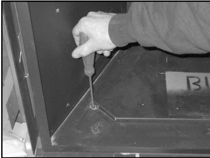
Figure 2: Removing floor shield.
