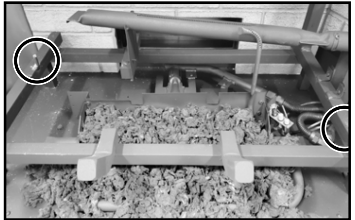
Figure 21: First log positioning pins.
