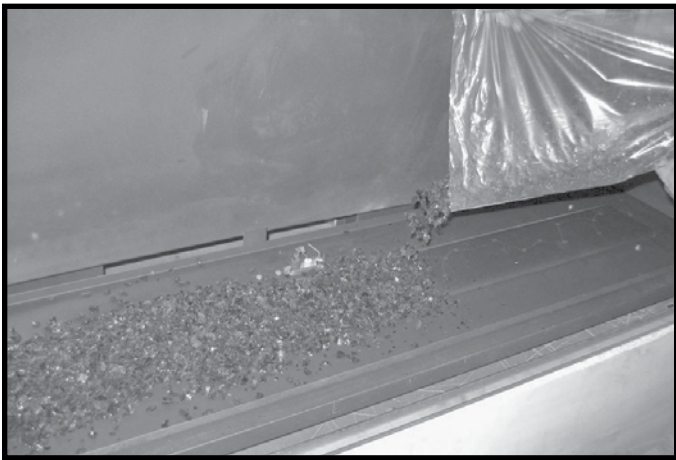
Figure 5: Applying glass media.
