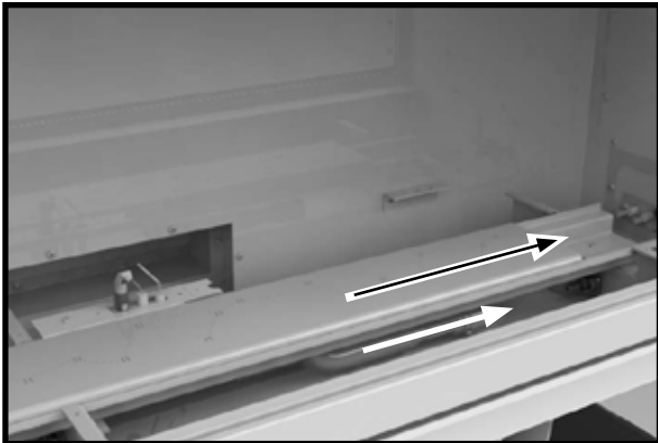
Figure 4: Installing right burner.
