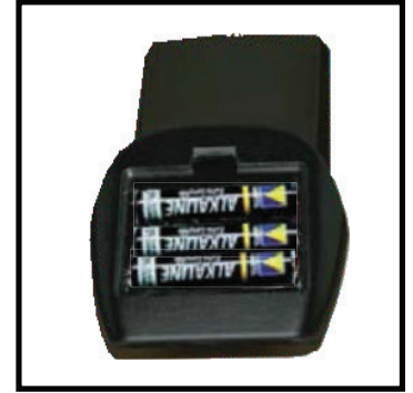
Figure 56: Proflame 2 remote battery compartment.
