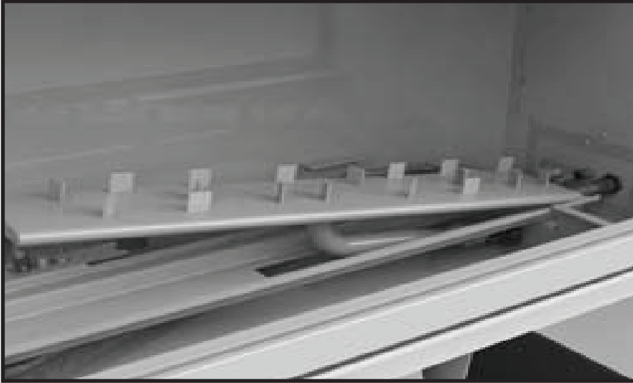
Figure 1: Burner tray installation.
