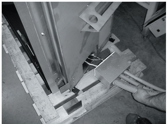
PULL OUT CONTROL ASSEMBLY
