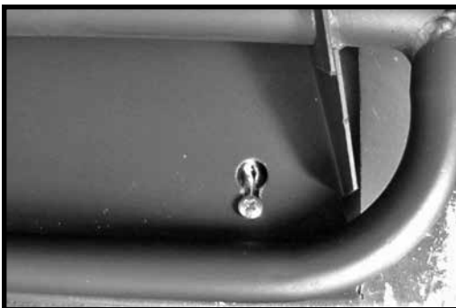
Figure 2: Attaching burner to floor of fireplace.
