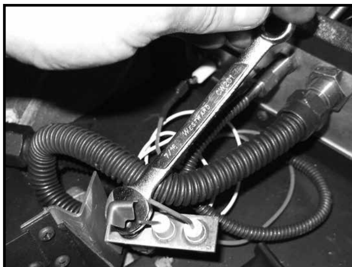
Figure 24: Loosening the pilot head.
