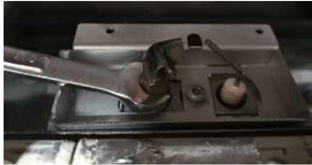
Figure 1: Loosen Pilot Head - PSE.
