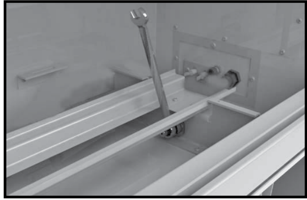
Figure 2: Removing the orifice.
