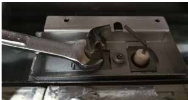
Figure 1: Loosen Pilot Head - PSE.
