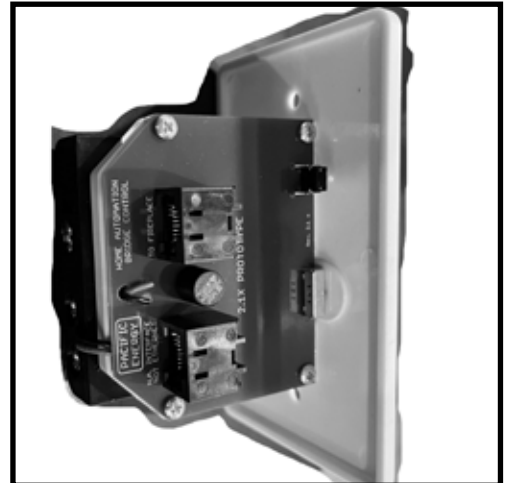
Figure 34: Basic wall switch - interface side.
