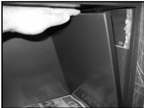
Figure 63: Removing the side panel.
