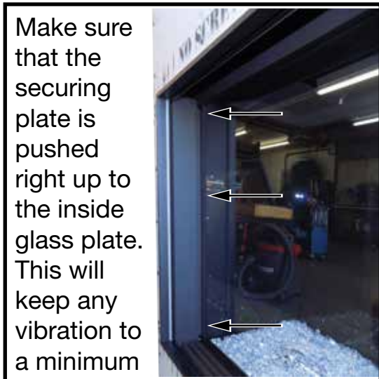
Figure 49: Position securing plate up against the inside glass plate.
