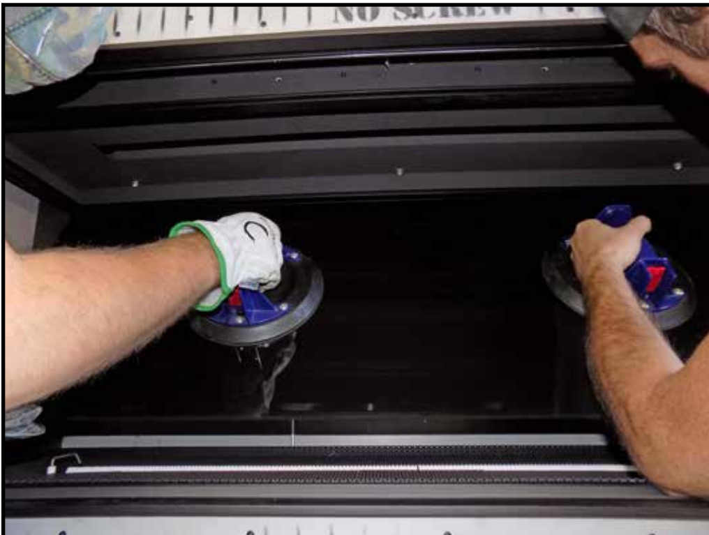
Figure 33: Insert top end of rear black glass plate first.
