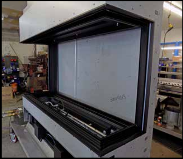
Figure 32: Rear wall before black glass sheet installation.
