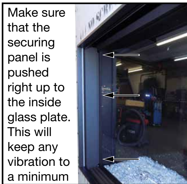
Figure 50: Position securing panel up against the inside glass plate.
