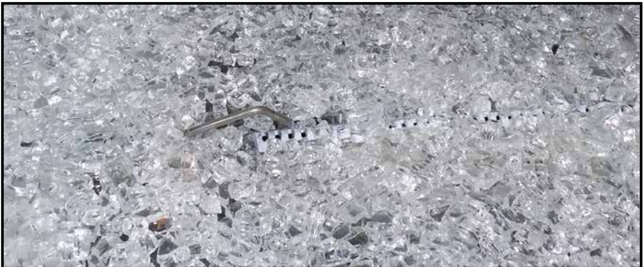
Figure 42: Exposed holes beneath the igniter.
