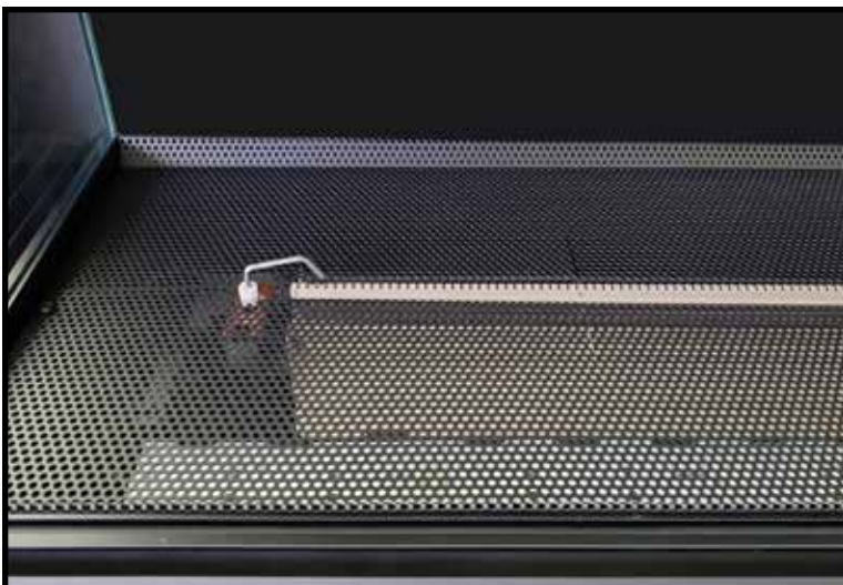
Figure 38: Burner tray in place.
