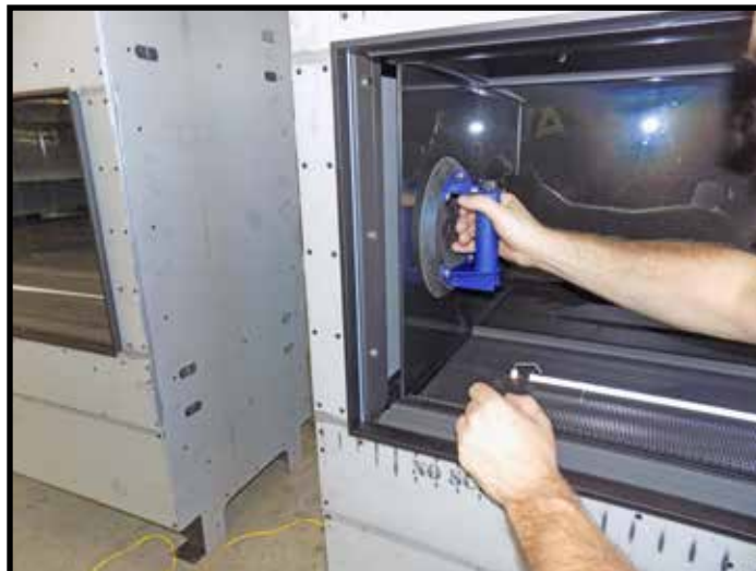
Figure 31: Insert bottom end of side black glass plate.
