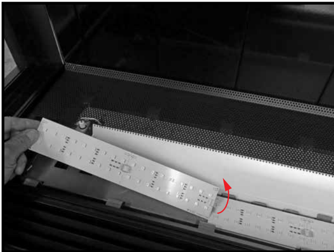
Figure 60: LED strip removal.
