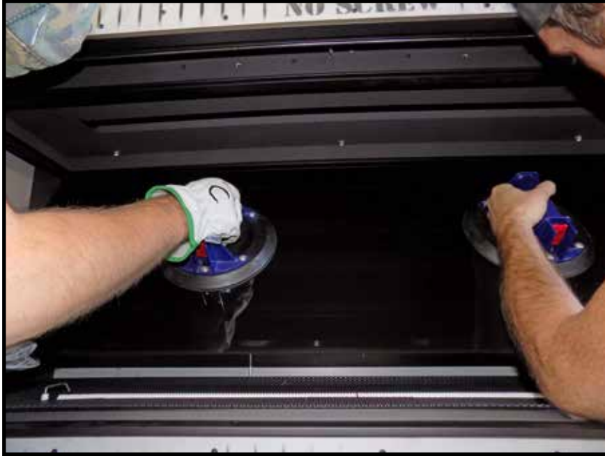
Figure 32: Insert top end of rear black glass plate first.
